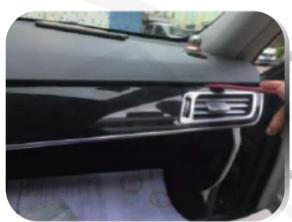
6. Pry the top buckles from the air conditioning vent. (Note: Ensure the vent is securely fixed when prying the buckles).
