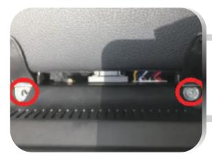
11. Attach the Android monitor to the stand, remove the screw cover, and lock the screws.
