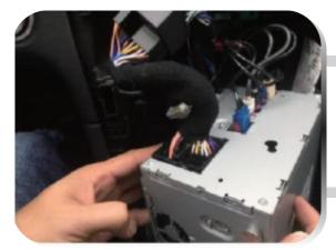
8. Disconnect the power harness from the NTG Unit and connect it to the Android harness.
