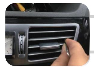
4. Pry the buckles on the right side of the air conditioning vent.
