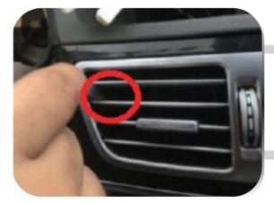
3. Pry the buckles on the left side of the air conditioning vent.
