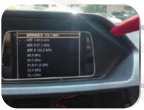
2. Carefully pry out the frame of the original screen and remove the fixing screws.
