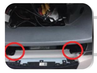
7. Remove the left and right fixing screws of the original NTG Unit.
