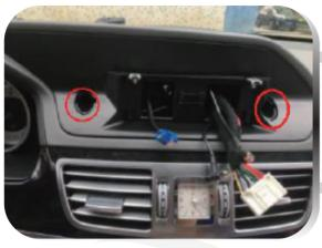
9. Assemble the Android screen stand securely onto the original dashboard and route the cables properly.
